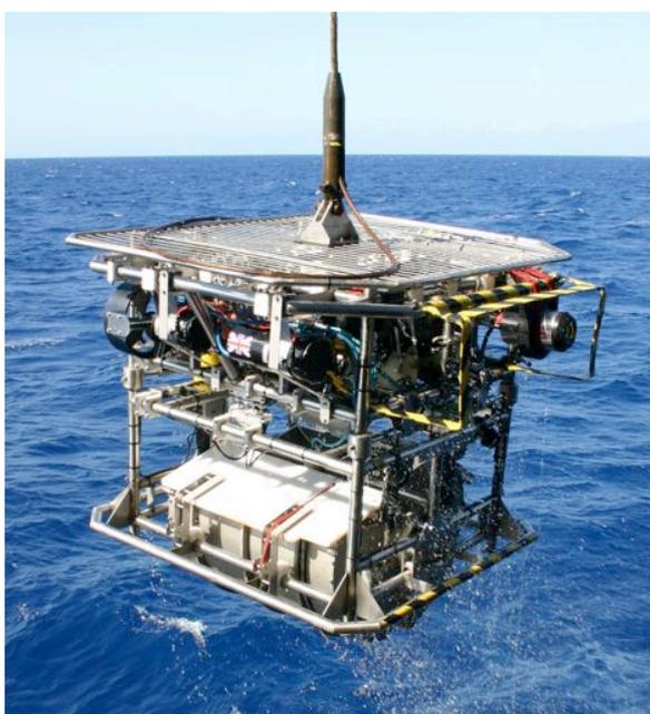
**Figure 3: The *HyBIS* ROTV being deployed from the RRS *James Cook*.**
